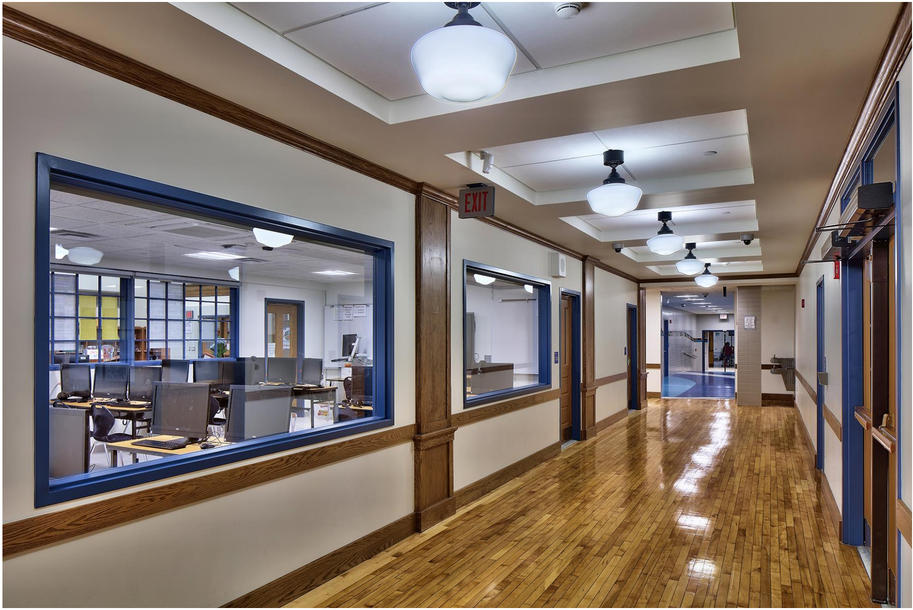
A “Legacy Corridor” within the original 1920 building was created by restoring original hardwood floors, wood trim, decorative column enclosures & providing Schoolhouse light fixtures
